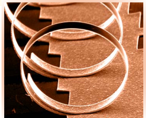
Released Cantilevers after Thermal Annealing Processed by Automegasamdri®-915B, Series C Nicolas André, Université Catholique de Louvain, Belgium
